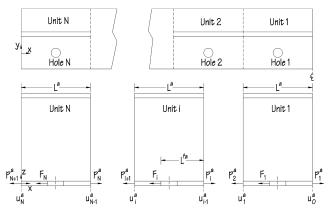
Fig. 8 Free-body diagram of Z-shaped aluminum beam.
