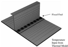
Fig. 16 Eight-unit fastened aluminum/composite assembly model.
