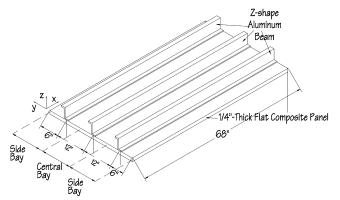
Fig. 1 Test article configuration.
