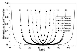
Fig. 27 Fastener-load transfer distribution for different fastened lengths.
