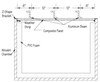
Fig. 5 Configuration of environment chamber with test article (side view).
