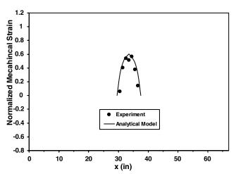
Fig. 25 Mechanical strains comparison between tests and analytical model for 8-fastener setup (7-in. fastened length).
