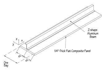
Fig. 7 One bay of aluminum/composite assembly test article.
