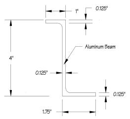
Fig. 2 Dimensions of cross section of Z-shaped aluminum beam.
