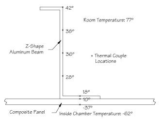
Fig. 18 Average temperature distribution of tests.
