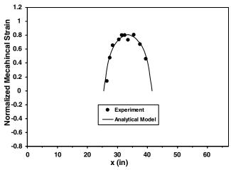
Fig. 24 Mechanical strains comparison between tests and analytical model for 16-fastener setup (15-in. fastened length).
