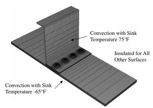
Fig. 15 Thermal finite element model of aluminum/composite assembly with four units.
