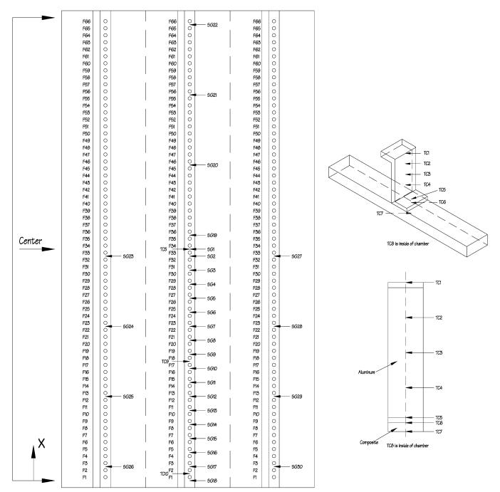
Fig. 3 Thermocouple and strain-gauge locations for the 66-fastener configuration with 10 thermocouples and 30 strain gauges.
