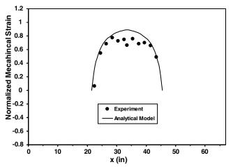
Fig. 23 Mechanical strains comparison between tests and analytical model for 24-fastener setup (23-in. fastened length).
