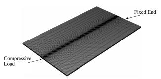
Fig. 13 Mechanical finite element model of flat composite panel with 20 units.
