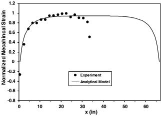
Fig. 20 Mechanical strains comparison between tests and analytical model for 66-fastener setup (65-in. fastened length).
