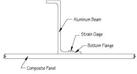
Fig. 11 Location of strain gauge.
