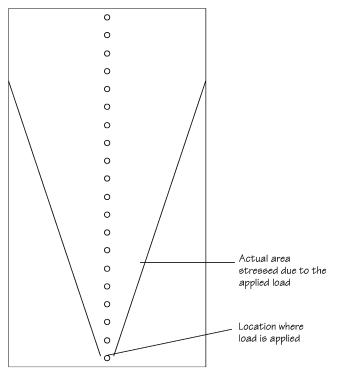
Fig. 10 Area influenced by external load in the wide composite panel.
