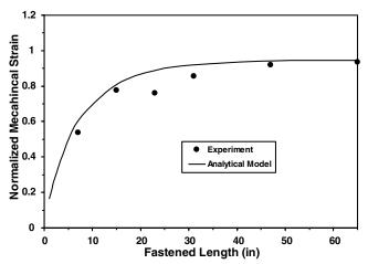
Fig. 26 Peak mechanical strains comparison between tests and analytical model for different fastened lengths.
