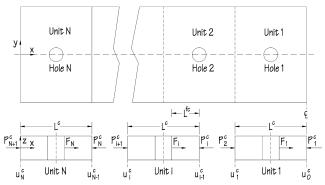
Fig. 9 Free-body diagram of flat composite panel.
