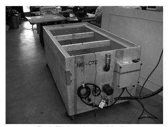
Fig. 4 Wooden environmental chamber.
