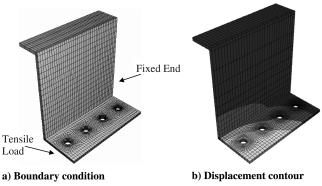
Fig. 12 Mechanical finite element model of Z-shaped aluminum beam with four units.
